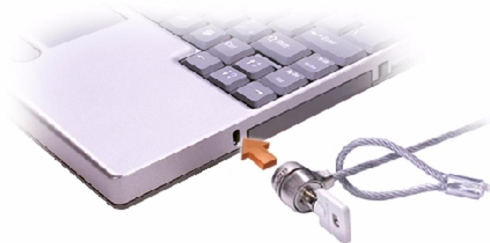
The slot lets you attach a commercially available antitheft device to the computer. Complete
